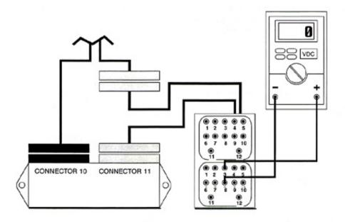
The adjustment of the CMP sensor will effect fuel ratios and ignition timing over the full operating range.
